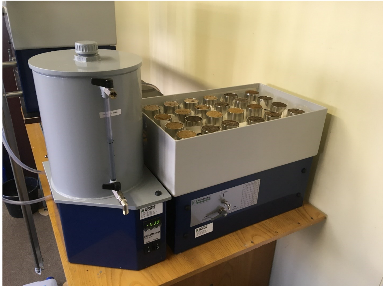
Fig. 1. Determination of the soil water retention curve (SWRC) using sand box and sand/kaolin box devices.
